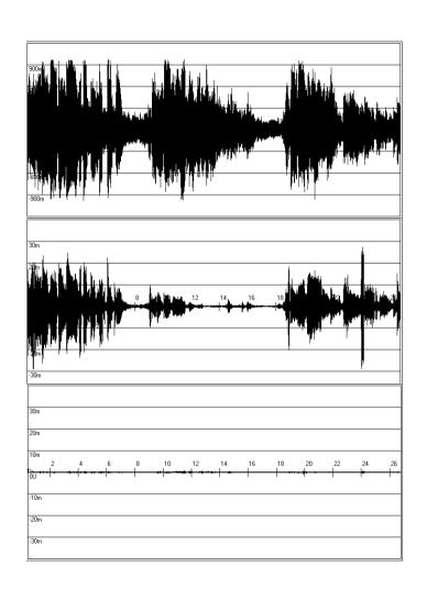
With a **0.1 ppm** rate mismatch, delay would be off by 1usec within 10seconds:
