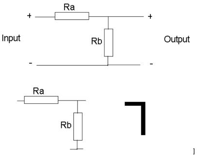
Notice how the two resistors (if you ignore the common wire to input and output) look like an upside-down "L", hence the name. The idea of the L-Pad is that the input side (amplifier or other circuitry) always sees an 8 ohm load if the output is an 8 ohm load, but less signal comes out of the output than if the L-Pad wasn't used.
